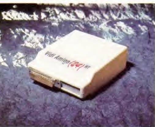
The Vidi 24 just plugs straight in to the parallel port of your Amiga
